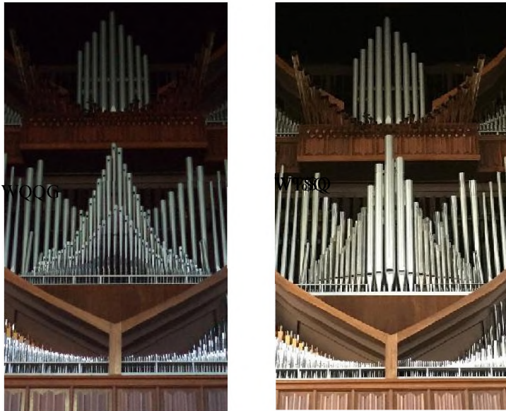
Figure 13. Left, the Harmonics V in front of the Swell box (Möller Organ). Right, the 8' Flûte harmonique in front of the Swell box (Reuter Organ).
