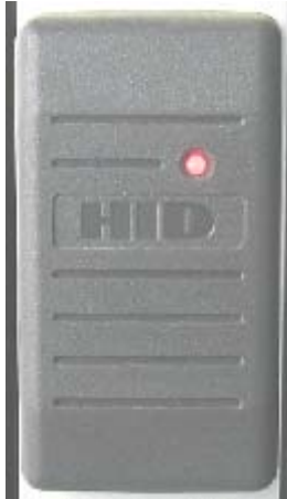
Figure 2-15 Bi-color LED in a Security Device
